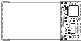
The 680 chip supports operation of the PCI bus at 32 bits, 33 MHz. The adapter may be used in either a 3.3V or 5V PCI signaling environment.
