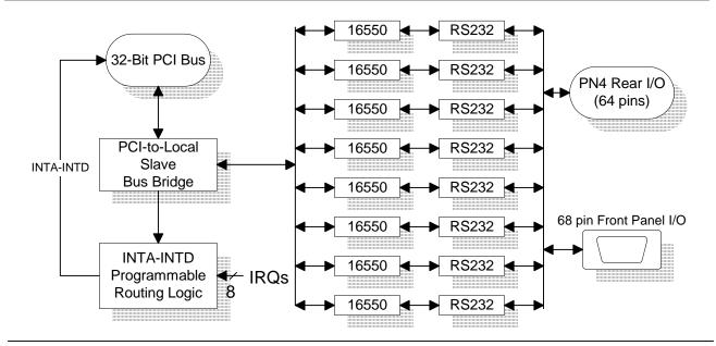
The Technobox 8-Port Async Communication adapter provides eight 16550-based UARTs using RS232 signaling levels.
