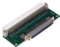
4400 SCSI Paddle Card for LVD rear I/O. Used with P/N 3145 and 4703 for rear I/O SCSI access.
