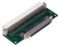
2699 Rear I/O paddle card for VMEbus P2. Used with P/N 2044 for rear I/O SCSI access.
