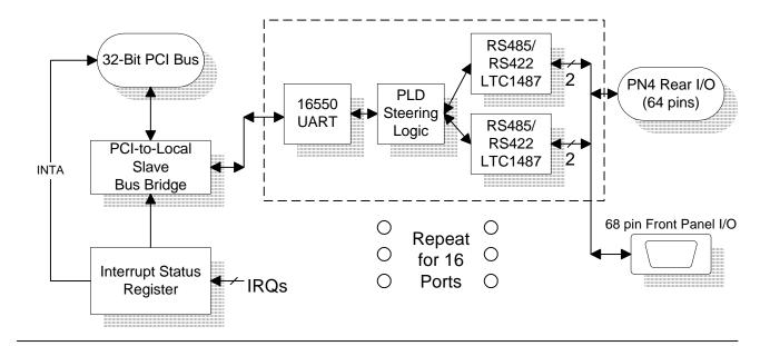
The 16-Port Async Communication adapter provides sixteen 16550-based UARTs using RS422 or RS485 signaling levels.
