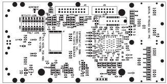
vided and are located per the VITA 20 conduction cooling specification, but this is not a conduction-cooling capable board. The anti-fretting holes at the rear behind PN2/PN4 and holes along the edge of the board for the secondary thermal interface are only provided for this purpose.
