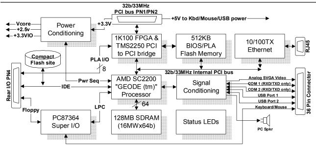
This board is a Processor PMC (PrPMC) implementing an x86-based PC architecture on a single-wide, standard height PMC form factor. This delivers a complete x86 platform with comprehensive I/O support, a 10/100-TX Ethernet interface, and disk access (both floppy and IDE drives). The board features an on-board hard drive using Compact Flash.
