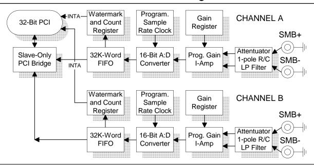
The Technobox 2-channel, 16-Bit Analog-to-Digital converter board features two independent Delta-Sigma A:D converter channels.
