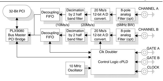
The 2-channel, 12-bit, 10Ms/s A:D converter provides a high performance data acquisition system on a single-wide PCI Mezzanine Card form-factor.
