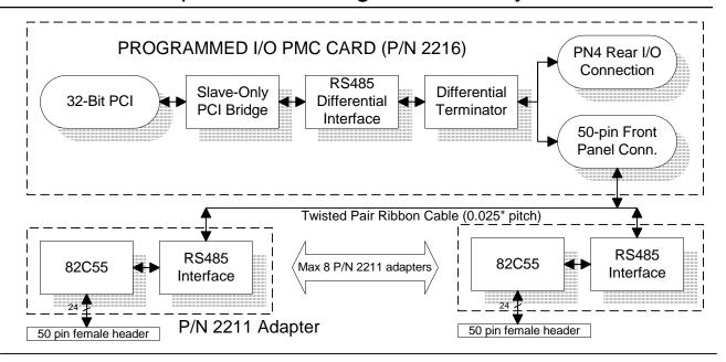
The Technobox 82C55 Digital I/O subsystem provides up to 192 points of 82C55-based digital I/O accessible from a single PMC slot.
