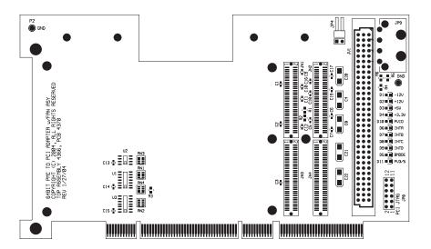
signaling level (either 3.3V or 5V), and clock speed — are transferred directly from the PCI edge fingers to the installed PMC. For applications requiring dissimilar PCI bus and PMC signaling, a bridged version of this board (either P/N 3673 or 4352) is available. All of these products use the same optional P/N 3675 fan assembly for forced-air cooling of installed PMCs.
