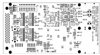
32-bit data bus is shared between the ALTERA and the PCI interface devices. The SRAM address is driven by ALTERA outputs. This technique allows a variety of memory architectures for the SRAM: single-port SRAM, dual-port SRAM, one or more FIFOs, and even linked list structures for more complex applications.
