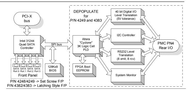
The "Versatile" Serial ATA controller provides four 1.5Gb/s links on a PMC front panel. Additional features are provided for rear I/O as described below.
