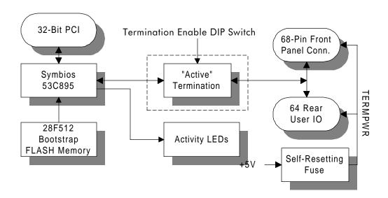
The ULTRA2 SCSI PMC adapter interfaces a host board PCI bus to a standard SCSI interface via a Symbios 53C895 controller, using either single ended or Low-Voltage Differential signaling.
