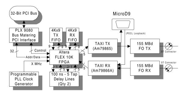
The Reconfigurable 155 Mb/s Fiber Optic (FO) PMC provides a means for implementing Fiber Optic interfaces for FDDI and other Fiber Optic standards having unusual requirements not supported by standard chipsets.
