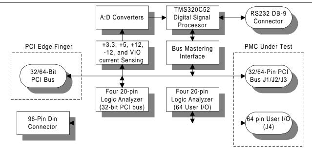
The Advanced PMC to PCI adapter is an engineering tool which permits development of a PMC card in a standard Personal Computer PCI slot.
