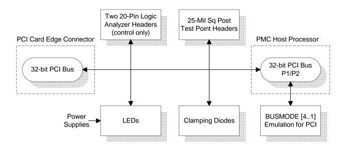
The Technobox PCI to PMC Adapter permits operation of a standard 32-bit PCI card in a PMC slot. It provides a migration path for standard PCI board suppliers to port their products to a PMC form factor. As the PMC equivalent board is developed, software development/migration can proceed with the original PCI board operating in a PMC environment. Also, developers can evaluate product performance in a PMC environment before committing to a PMC conversion effort.
