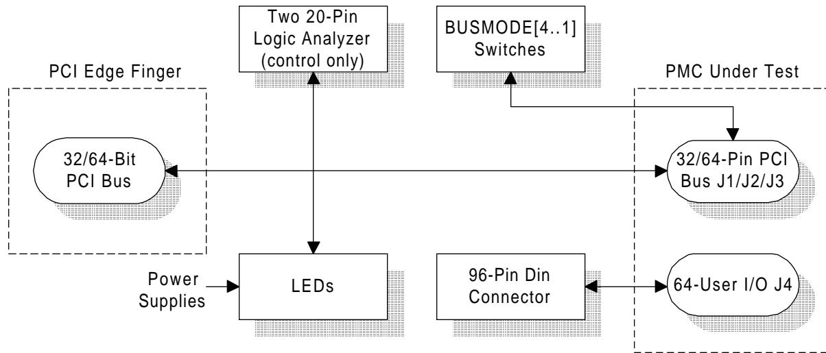
The PMC to PCI Adapter is intended for engineering test environments where demonstration in a PCI-compliant system using standard PCI boards is desired.
